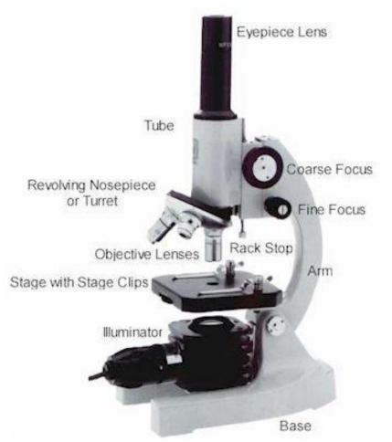
Stage: The flat platform where you place your slides. Stage clips hold the slides in place.
